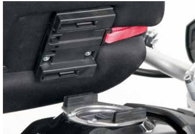
Underside of a tank bag with matching counterpart to the tank ring
