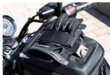
Practical Velcro fastener for attaching gloves, such as at tollbooths or fuel stations
